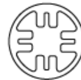
Base Footprint Circular base pattern requiring four (4) 1/2" anchor bolts
